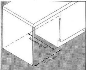
It is recommended that a 650mm wide worktop is used, but in some situations a 600mm worktop will be satisfactory and allow adequate space for the Easy-Fit hinge and fascia to be fitted in the correct line (check the depth of the appliance to determine which will be suitable). If extra ventilation is required (see manufacturers recommendations), a grille may be installed in either the plinth or the back of the work surface.
