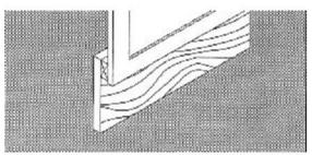
Where the Easy-Fit hinge is to be used for a slim-line fridge, freezer or dishwasher, a spacer will be required to attach the plinth to the fascia, to open in one action.
