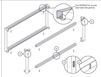
Locate 4 x R7712 profiles and attach to connecting blocks using black coated screws.
