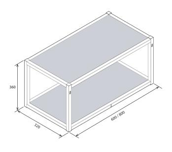
**NOTE:** Supplied with FISCHER DUOPOWER dowels for wall fixing. Important, please assess wall construction and determine wall fixings to suit.
